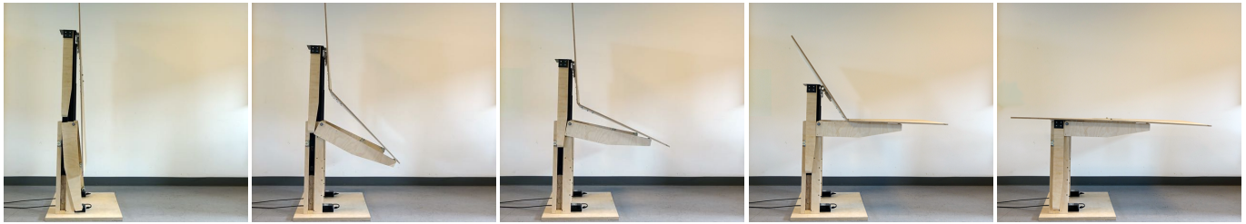
Figure 4. Five example positions of the dynamic surface prototype. Vertical movement from the linear actuators are translated into a pivoting movement that lifts the plywood arms and lifts the hinged table surfaces.
